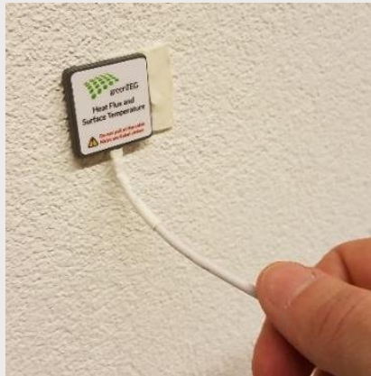
Figure 4: How to demount the sensors
